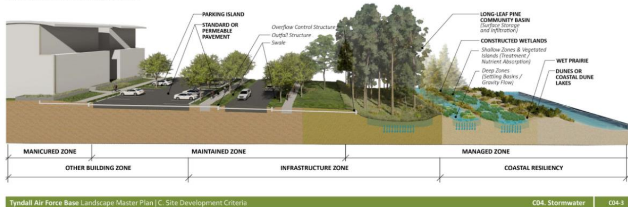
Figure 14 Stormwater Treatment Train (Source: Tyndall AFB Landscape Master Plan Exhibit C04 )
